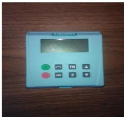
**Figura 2.40:** Basic Operator Panel
